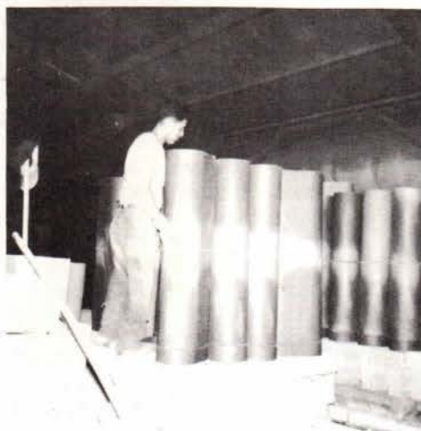
Pipe being stacked for entry into baking oven.
