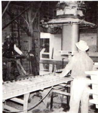
Machine is also used for molding clay pipe.
